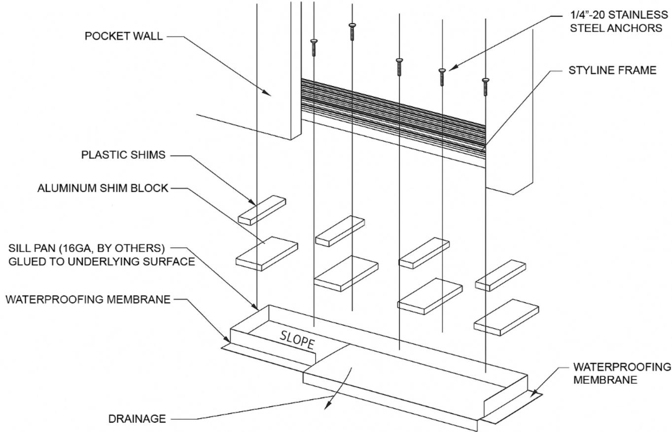
**Step 3:** Using Schnee SM7713 MS Permathane, glue sliding door sill and anchor in place (anchors are not always necessary), You may now begin to Plum, Level and Square the system into the opening.
